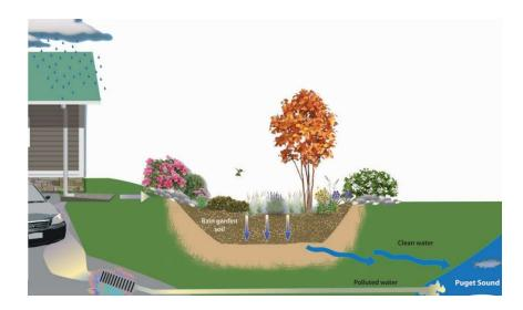
Figure 2.4 An example of how a rain garden functions and prevents runoff from entering the lake, from <a href="http://kitsapcd.org/programs/raingarden-lid/rgbasics">http://kitsapcd.org/programs/raingarden-lid/rgbasics</a>.
