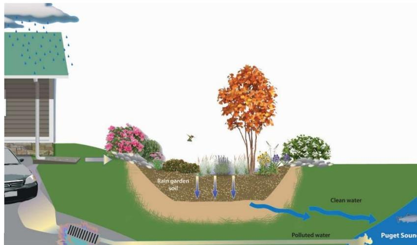
Figure 2.4 An example of how a rain garden functions and prevents runoff from entering the lake, from <http://kitsapcd.org/programs/raingarden-lid/rgbasics>.
