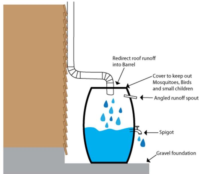
Figure 2.2 Image of a rain barrel system adapted from
